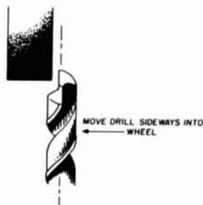
fig. 9. Normal drills can be converted to a brass grind by changing the rake angle at the tip. This alleviates problems with cracking and chipping when drilling plastics.
