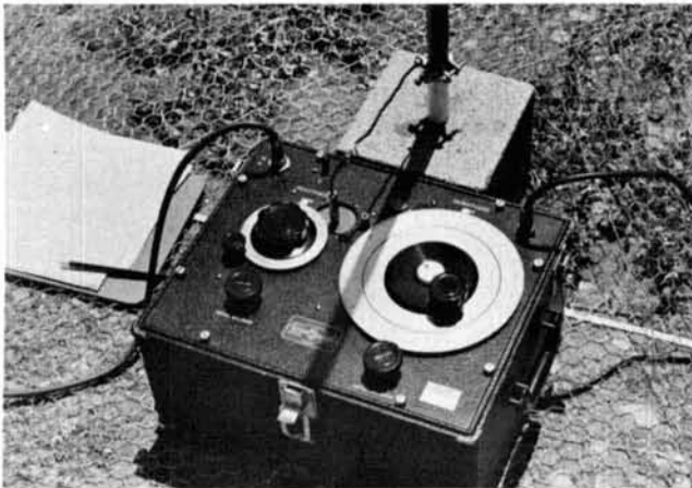
A GR-916A rf-impedance bridge was used to make the impedance measurements. The chicken-wire mesh can be seen laid on top of the ground.
